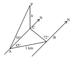
An aeroplane is sighted simultaneously from two stations A and B, B being one kilometre north-east of A. To the observer at A the aeroplane appears due north at an elevation of 34°; to the observer at B it appears in a direction N72°W.
