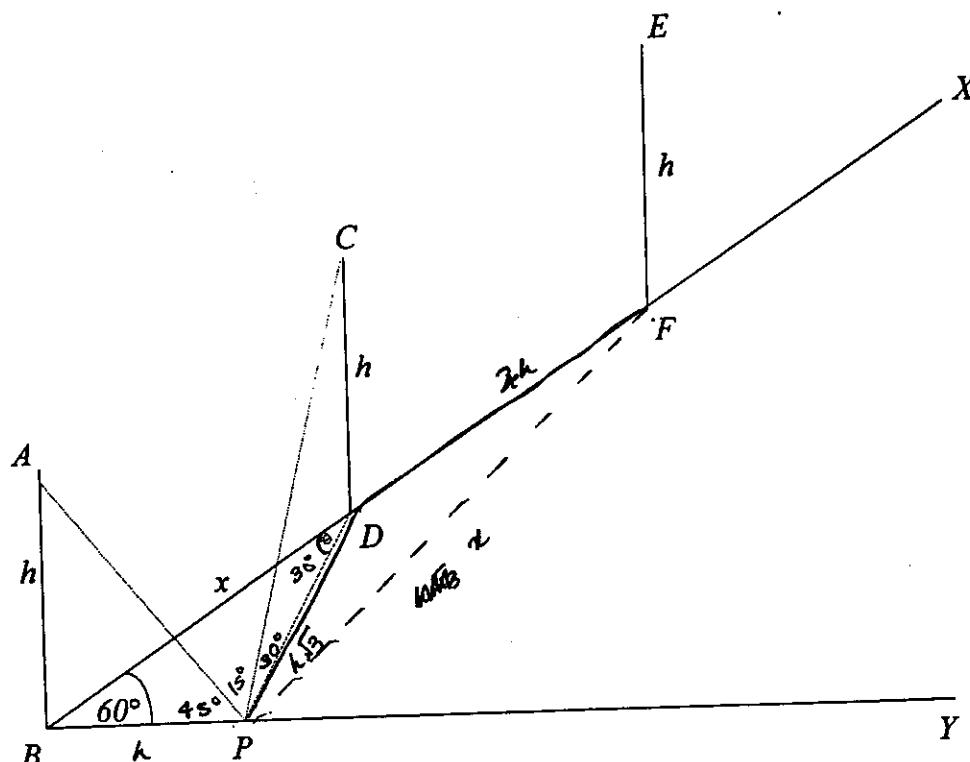
In the above diagram,  $BX$  and  $BY$  represent two roads intersecting at an angle of  $60^\circ$ . On the road  $BX$  are situated three telegraph poles  $AB$ ,  $CD$  and  $EF$ , all of equal height, the same distance,  $x$  metres, apart (i.e.  $BD = DF = x$ ).  $P$  is a point on the road  $BY$  and the angles of elevation of  $A$  and  $C$  from  $P$  are  $45^\circ$  and  $30^\circ$  respectively.
