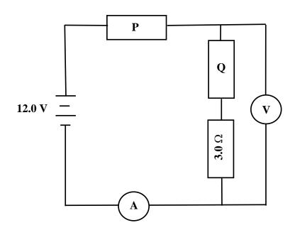
The reading on the ammeter is 1.5 A. The reading on the voltmeter is 6.75 V.
