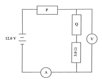
The reading on the ammeter is 1.5 A. The reading on the voltmeter is 6.75 V.
