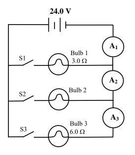
**Bulb 1** has a resistance of 3.0  $\Omega$ . **Bulb 3** has a resistance of 6.0  $\Omega$ . When all three switches are closed (on), **ammeter A**<sub>1</sub> has a reading of 18.0 A.
