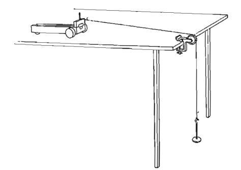
The trolley is released from rest and the time taken to travel 0.4 m is recorded on a stopwatch as taking 0.76 s. The total mass of the mass-carrier is 50 g.
