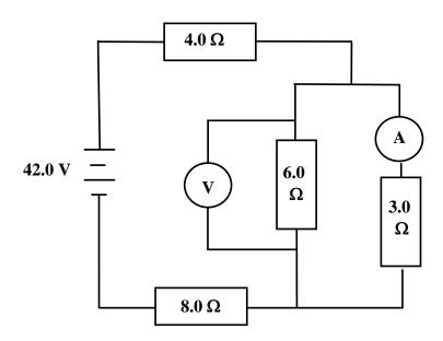
Determine the total current in the circuit. (a) 2 ..... ..... ..... ..... Determine the reading on the voltmeter. (b) 1 ..... ..... Determine the reading on the ammeter. (c) 1
