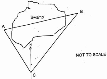
The diagram shows two points A and B on opposite sides of a crocodile infested swamp. From a point C a surveyor notes that the bearings to A and B are 340° and 036° respectively. The distances AC and BC were then measured and found to be 180 metres and 212 metres respectively.
