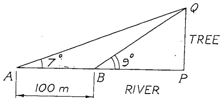
The diagram above was sketched by a surveyor, who measured the angle of elevation of a tree top on the other side of the river to be  $7^\circ$  at the point  $A$ . At point  $B$ , 100metres directly towards the tree from  $A$ , the angle of elevation was  $9^\circ$ .
