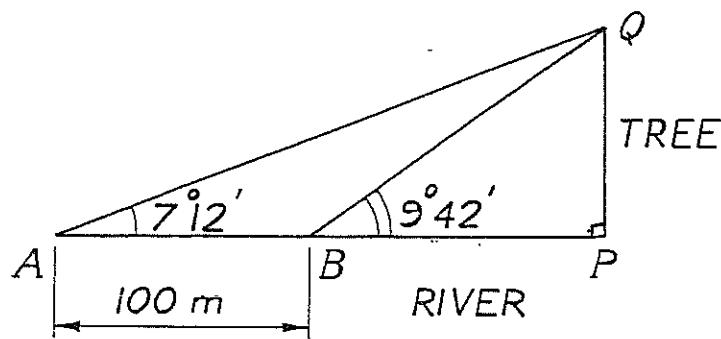
The diagram above was sketched by a surveyor, who measured the angle of elevation of a tree top on the other side of a river to be  $7^\circ 12'$  at the point A.
