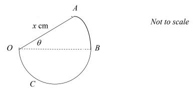
The cam's cross-section consists of a semi-circle *OCB* and the sector of a circle *OAB* of centre *O* with a radius of *x* cm and with an included angle  $BOA = \theta$ .
