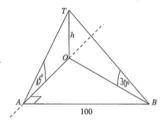
A surveyor stands at a point A, which is due south of a tower OT of height h m. The angle of elevation of the top of the tower from A is 45°. The surveyor then walks 100 m due east to a point B, from where she measures the angle of elevation of the top of the tower to be 30°.
