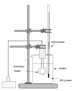
The immersion heater provided 75.7 kJ of heat which raised the temperature of the water in the beaker from  $25^{\circ}$ C to  $85^{\circ}$ C.
