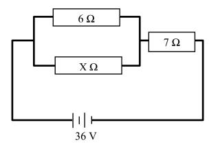
A current of 0.5 A flows through resistor X.
