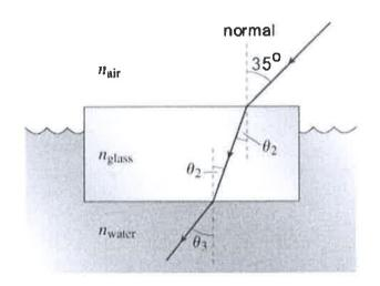
Calculate the angle of refraction,  $\theta_2$ , as the light passes from air to (a) glass.
