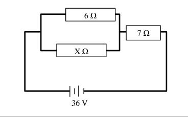
A current of 0.5 A flows through resistor X.
