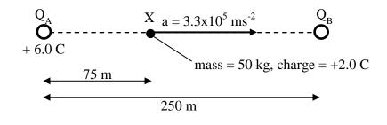
When it is released, the charge at X has an acceleration of  $3.3 \times 10^5$  ms<sup>-2</sup> to the right.
