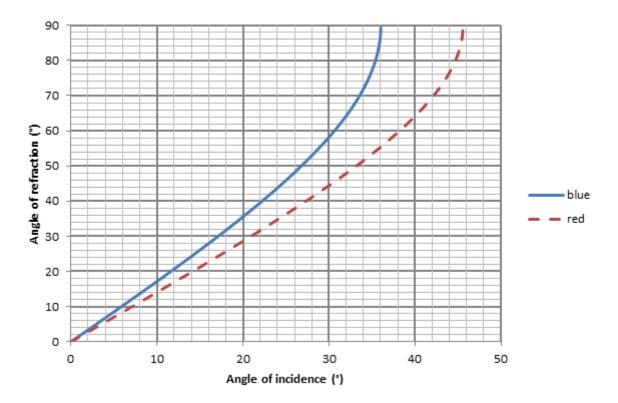
(a) Use the graph to determine the critical angle for blue light in Medium X. 2
