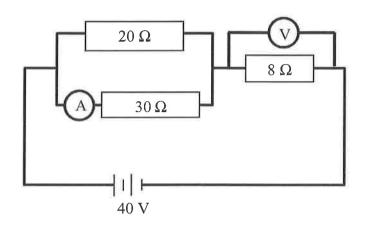
(a) Determine the total resistance of the circuit.  $R_{II} : \frac{1}{R_{II}} = \frac{1}{20} + \frac{1}{30} = R_{II} = 12 \times 10 \text{ mk.}$   $R_{+otal} = 8 + 12 = 20 \times 10 \text{ mk.}$
