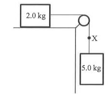
The blocks are connected by a light, inextensible string over a frictionless pulley. The 2.0 kg block is resting on a smooth horizontal surface.
