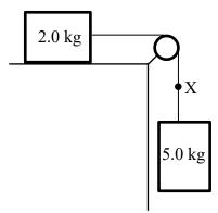
The blocks are connected by a light, inextensible string over a frictionless pulley. The 2.0 kg block is resting on a smooth horizontal surface.
