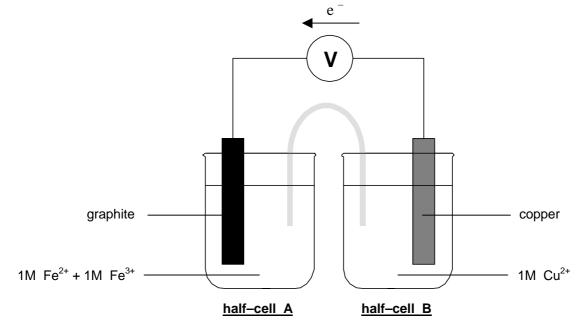
After operating for several hours chemical changes are evident. The reaction occurring in half–cell A is...  $Fe^{3+}_{(aq)} + e^{-} \rightarrow Fe^{2+}_{(aq)}$
