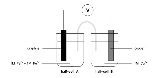
After operating for several hours chemical changes are evident. The reaction occurring in half–cell A is...  $Fe^{3+}_{(aq)} + e^{-} \rightarrow Fe^{2+}_{(aq)}$
