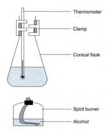
Methanol, ethanol and 1-propanol were burned in separate spirit burners and used to heat a container of water. The volume of water heated by each alkanol was 100.0 ml.
