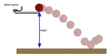
The horizontal distance travelled from the edge of the table was marked on the floor and measured with a metre rule.
