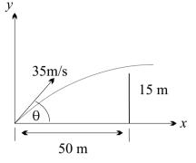
The diagram above shows a stone thrown with a velocity of  $35 \,\mathrm{m/s}$  at an angle  $\theta$  so that it just clears a 15 m high wall that is 50 m from the origin on the same horizontal plane.
