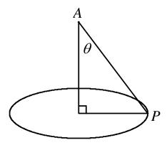
The particle *P* rotates with angular velocity  $\omega$  radians per second in uniform circular motion radius 8cm in the horizontal plane, and has a semi-vertical angle  $\theta$  with point *A*.
