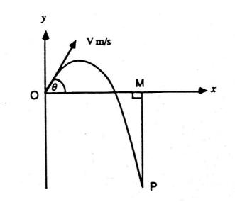
A projectile is fired from a point O with initial speed V m/s at an angle of elevation of  $\theta$ . It is subject only to the force of gravity, resulting in a constant downward acceleration of magnitude g m/s<sup>2</sup>.
