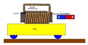
(c) Lenz's law states: "The effect of an induced emf is such as to oppose the change in magnetic flux that causes the induced emf." Analyse your prediction in part (b) using Lenz's law.
