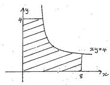
The area enclosed by the curve xy=4, the x axis and y axis, and the lines y=4 and x=8, is rotated about the y axis.
