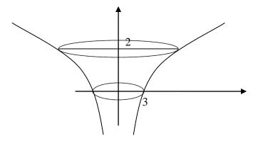
$$Vol = \pi \int_{0}^{h} (2 + e^{y})^{2} dy = \pi \left[ 4 + 4e^{y} + \frac{1}{2}e^{2y} \right]_{0}^{h} = \pi \left[ 4h + 4e^{h} + \frac{1}{2}e^{2h} - 4 - \frac{1}{2} \right]$$
