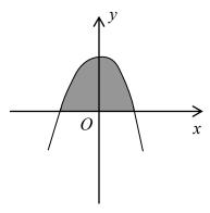
The shaded region lying between the curve  $y = 4 - x^2$  and the x - axis is rotated about the x - axis.
