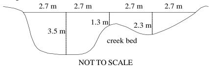
By using Simpson's rule twice, find an approximation for the area of this cross-section of the creek.
