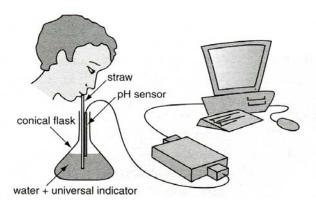
The students used the pH sensor with the datalogger, setting the *x*-axis as time and the *y*-axis as pH. Distilled water was placed in a dishwasher-cleaned conical flask. Universal indicator was added to the distilled water and it turned dark green.
