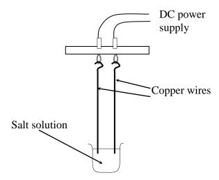
When the power was switched on the student observed that the wires were weakly repelled from each other. The student then decided to try to modify the set-up so that the wires will now be attracted to each other and also to attempt to increase the size of the force acting. Which of the following combinations of changes could the student make to the set-up to be sure they will achieve the desired result?
