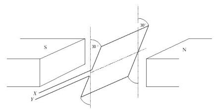
X is connected to the positive terminal of a power supply, and Y is connected to the negative terminal. The coil is set in the position shown and viewed from the front near X and Y. Which of the following will occur when the power supply is turned on?
