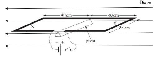
When the switch is closed, a current of 30 amperes flows through the coil. Which of the following would prevent the coil from starting to rotate when the switch is closed?
