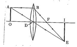
The lens diagram shows two rays of light A-B-E and A-D-E which meet at E. OA is the object and IE is the image and they are both vertical.
