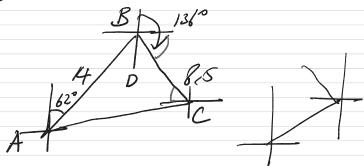
b) use cosine rule  $AC^{2} = 14^{2} + 8.5^{2} - 2 \times 14 \times 8.5 \text{ costab}$  AC = 18.27 AC = 18.27 AC = 18.27
