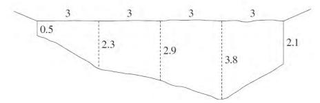
Use the trapezoidal rule with the five depth measurements to calculate the approximate area of the cross section.
