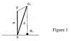
Figure 1 above shows the block is at  $H_1$  on the ground. The hoist rope, anchored at *E*, passes over pulleys at *F* and  $G_1$ , then reaches vertically downwards and is attached to the block.
