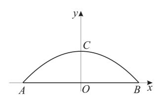
The diagram above shows the side view of a bridge. The level roadway AB lies on the x-axis, and the steel arch ACB is a parabolic arc with equation  $x^2 = -180(y - 45)$ . On both the x and y axes, one unit represents one metre.
