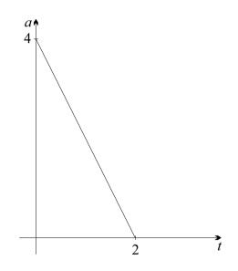
A particle is moving along the x-axis. The graph shows its acceleration  $a \text{ m/s}^2$  at time t seconds. Initially the particle has a velocity of -2 m/s. What is its velocity after 2 seconds?
