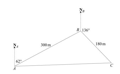
Dave flies a drone 300 metres from A to B on a bearing of  $062^{\circ}$ . It then changes direction to fly 180 m from B to C on a bearing of  $136^{\circ}$ .
