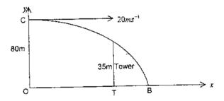
Assuming there is no horizontal acceleration and vertical acceleration is due to gravity the equations of motion for the particle are  $\ddot{x}=0$  and  $\ddot{y}=-g$ . The origin is the base of the cliff, O, and gravity,  $g=-10ms^{-2}$ .
