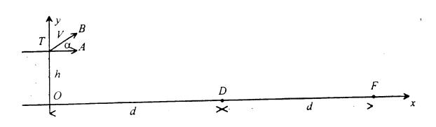
The equations of motion of both particles are  $\ddot{x} = 0$ ,  $\ddot{y} = -g$ .
