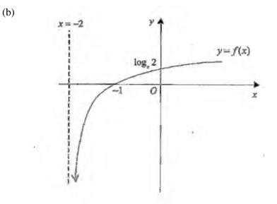
The diagram shows the graph of the function  $f(x) = \ln(x+2)$ .
