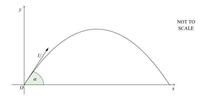
The equations of motion are  $x = Ut \cos \alpha$  and  $y = Ut \sin \alpha - \frac{1}{2}gt^2$ , where t is time in seconds. **Do NOT prove these results**
