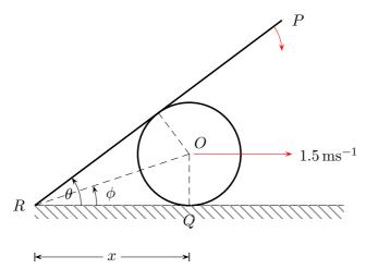
The disc rolls to the right with a constant speed of  $1.5 \text{ ms}^{-1}$ . As the disc rolls, the other end of the rod P commences its descent towards the ground.
