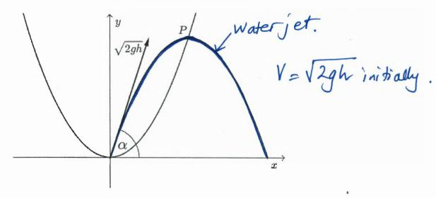
The equations of motion of a projectile fired from the origin with initial velocity  $V ms^{-1}$  at angle  $\alpha$  to the horizontal are:
