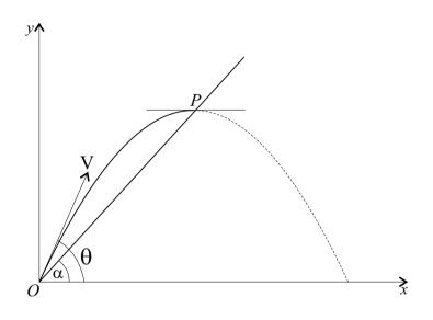
In the diagram above the point O is the foot of a plane inclined at an angle  $\alpha$  to the horizontal. A particle is projected with speed V from O at an angle of elevation  $\theta$  to the horizontal, where  $\theta > \alpha$ . It strikes the inclined plane at P, which is the vertex of the parabolic path of the particle. You may assume that this parabolic path has parametric equations  $x = Vt \cos \theta$  and  $y = Vt \sin \theta - \frac{1}{2}gt^2$ .
