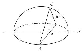
The solid shape above has a circular base of radius 3 units in the horizontal plane. Vertical cross-sections perpendicular to the diameter along the *x* axis are equilateral triangles as shown in the diagram.
