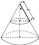
The particle P rotates with uniform velocity  $\omega$  radians/second in a horizontal circle on he outside surface of the cone and in contact with it.
