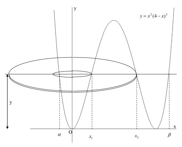
The region between x = 0 and x = 4 is rotated about the y - axis. The volume of the solid formed is found by taking slices perpendicular the the y - axis. The typical slice shown in the diagram is at a height y above the x - axis.
