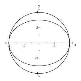
A straight line l parallel to the y axis intersects the x axis at N and the ellipse and the auxiliary circle at the points P and Q respectively.
