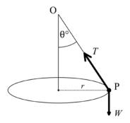
The tension in the rod is T newtons and the weight of P is W newtons. The radius of the circle is r metres.
