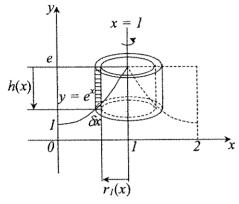
The typical cylindrical shell has radii  $r_1(x) = 1 - x$ ,  $r_2(x) = 1 - x + \delta x$ , and height  $h(x) = e - e^x$ . This shell has volume
