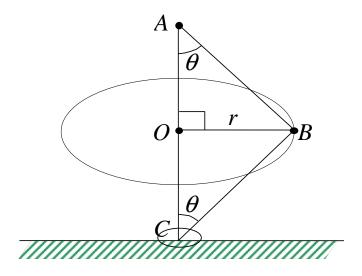
The joint at *B* has a particle of mass 2 kg attached. A small ring of mass 1 kg is smoothly joined to *BC* at *C* and can slide on the vertical rod below *A*. The ring rests on a smooth horizontal ledge at a distance  $\frac{\sqrt{3}}{2}$  m below *A*. The system rotates about the vertical rod with constant angular velocity 6 radians per second. Find:
