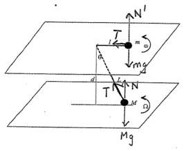
iii) Consider *m*: Vert: N' = mgHor:  $T = ml\omega^2$  – Equate (1) & (2)  $ML\Omega^2 = ml\omega^2$  $\frac{L}{l} = \frac{m}{M} \left(\frac{\omega}{\Omega}\right)^2$  –
