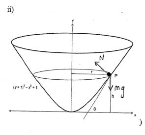
iii)  $H: N \sin \theta = mr\omega^{2} - (1)$  $V: N \cos \theta = mg - (2)$  $\therefore N = \frac{mg}{\cos \theta}$  $Sub - (1) \frac{mg}{\cos \theta} \sin \theta = mr\omega^{2}$  $\tan \theta = \frac{r}{1+h} \quad \frac{g \times \gamma}{(1+h)} = \gamma\omega^{2}$  $\therefore \omega^{2} = \frac{g}{1+h}$
