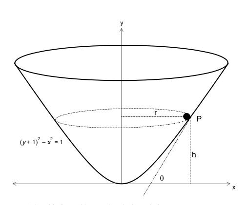
A smooth bowl is formed by rotating the hyperbola  $(y+1)^2 - x^2 = 1$  around the *y* axis.
