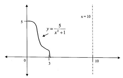
A circular flange is formed by rotating the region bounded by the curve  $y = \frac{5}{x^2 + 1}$ , the x axis and the lines x = 0 and x = 3, about the line x = 10. (All measurements are in cm)
