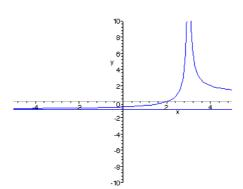
Vertical asymptote at x=3 and a horizontal asymptote at y=-1. Note that for x < 3 the graph is -f(x).
