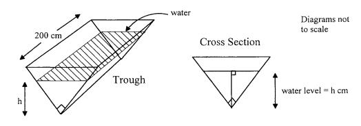
Water is flowing into the trough at the rate of  $12cm^3s^{-1}$ . Find the rate of change of the upper surface area of the water when the height of the water is 12cm
