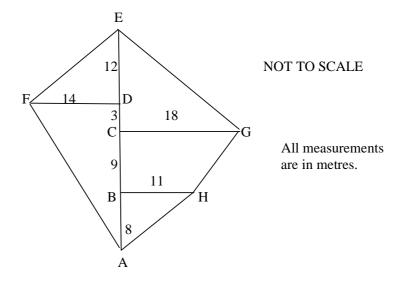
(i) What are the missing values of x and y in the offset survey from this field diagram?
