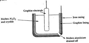
A mixture of aluminium oxide and cryolite is kept molten in a large iron box lined with graphite. This lined box acts as the cathode. Another graphite electrode is placed into the mixture. During the electrolysis, carbon dioxide gas forms at this electrode. Molten aluminium falls to the bottom of the box and is drained off.
