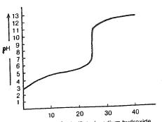
Volume (mL) of diluted sodium hydroxide added to 25.0mL of diluted acetic acid
