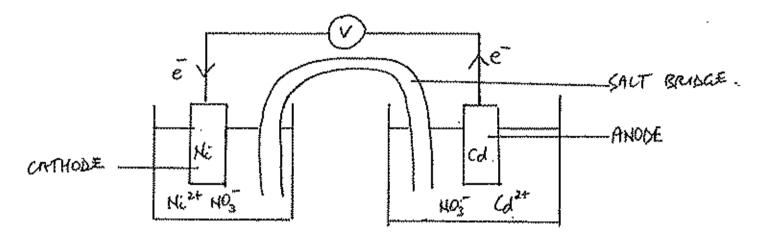
(b) Given that the standard reduction potential of the cadmium half cell is -0.4V, show on your diagram the direction in which electrons will flow in the external circuit of this cell.
