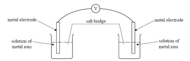
For each cell, the polarity of the electrodes and the voltage generated are recorded.
